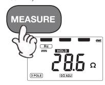
The FT6031-03 automatically checks the ground potential, checks the auxiliary grounding electrode, and measures the grounding resistance. The instrument also selects the optimal range for the grounding resistance, eliminating the need to switch ranges and enabling efficient measurement.
