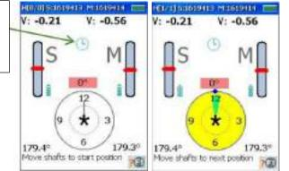
When the automatic data acquisition mode is active, the device waits for a stable shaft position, then automatically records the data and prompts you to move the shafts to the next position.
