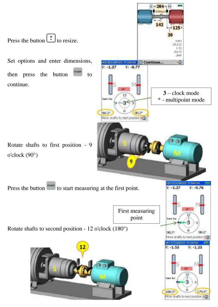
Press the button to start measuring at the second point.
