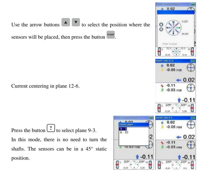
The color of the clutch symbols indicates the amount of misalignment. Green indicates when the residual offset is within tolerance. Black color for perfect results. Always stop machine offset when the residual offset is within tolerance. Don't try to reach zero.
