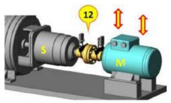
For adjustment in the horizontal direction, the sensors must be rotated 9 or 3 o'clock ( $90^{\circ}$  or  $270^{\circ}$ ).
