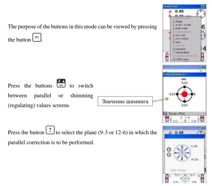
For in-plane correction, 9-3 sensors must be set to 9 or 3 o'clock.
