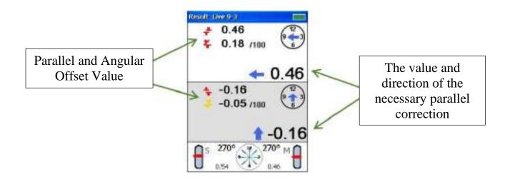
The blue arrows indicate the directions in which the movable machine must move in order to eliminate parallel displacement.
