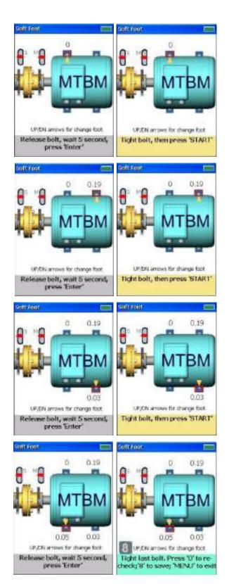
You can change the bolt selection sequence by manually selecting the bolt using the arrow buttons.
