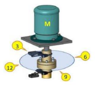
Electronic inclinometers cannot be used on vertical machines, so Manual Angle is set by default. Before you start measuring, you must specify the measuring points on the machine.
