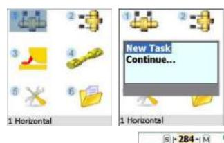
The measurement settings window will open with machine dimensions. Press the button to start editing dimension values.
