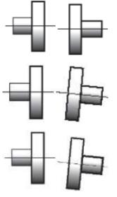
Parallel misalignment - the center lines of the two shafts, although parallel, do not coincide.
