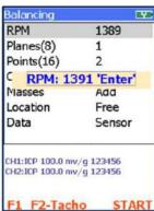
**Note.** If the actual RPM and the trim RPM differ by more than 5%, the device displays an error message.
